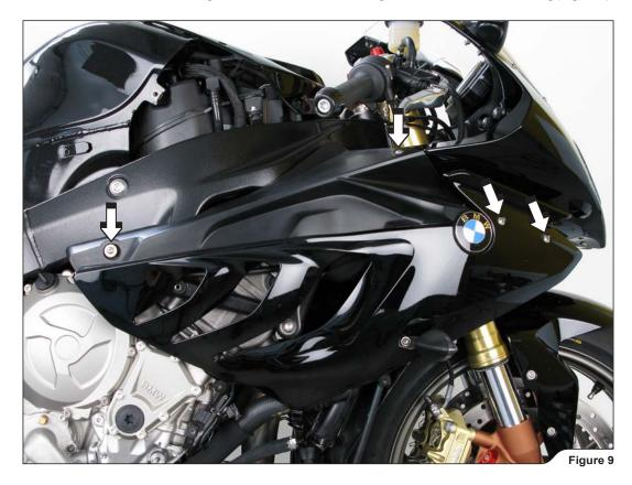
WARNING: disconnect the turn signal elecrical connectors during removal of the middle cowling (Figure 9)!
