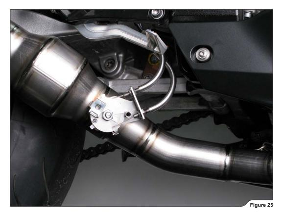
10. For street legal Racing and Evolution only: set the cable adjusters on the middle of the cable bracket, as shown. Tighten the cable adjusters nuts to a specified torque (Figure 26).
